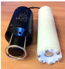
Figure 2: Underwater monitoring node: acoustic modem and measurement probe with the Gumstix inside the PVC housing.
