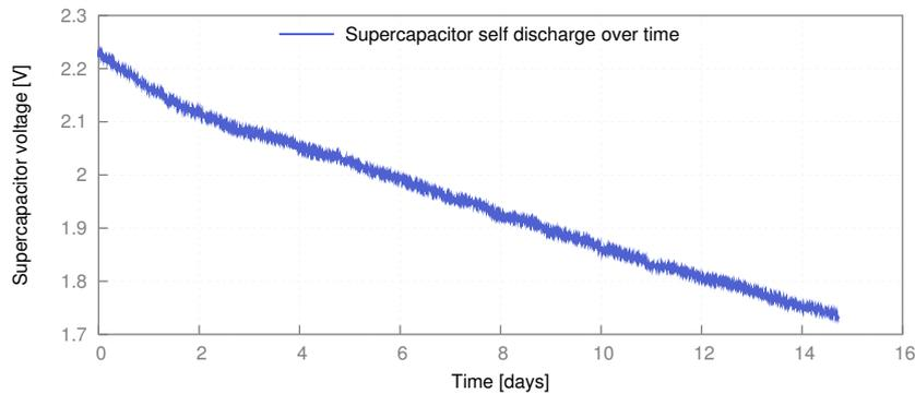
**Figure 1.3** Self discharge of a supercapacitor over time.
