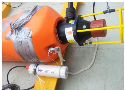
(c) CLAM cNode equipped with the WSENSE CO<sub>2</sub> sensor.
