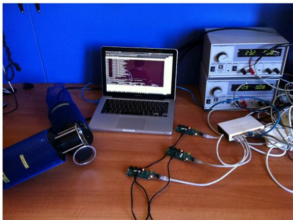
Figure 3: Laboratory testbed using the channel emulator and SUNSET running on different hardware platforms.
