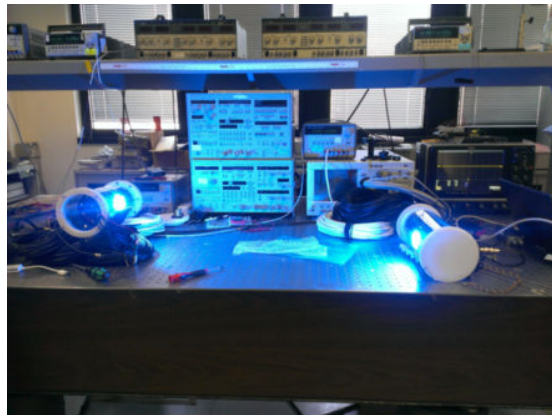
Figure 3: Laboratory experiments with two OptoCOMM modems during a file transmission.
