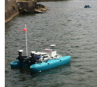
(a) Underwater monitoring node: Measurement probe with the Gumstix inside the PVC housing. (b) MARES AUV with acoustic modem. (c) INESC ASV with acoustic modem.
