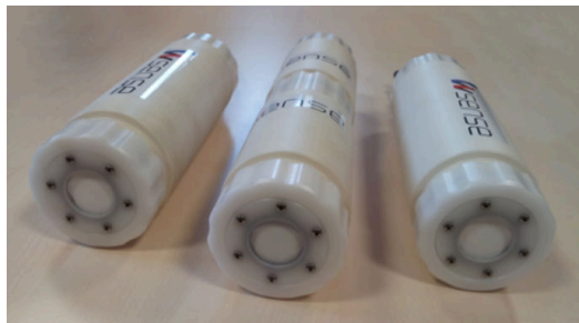
(a) Underwater monitoring node: Measurement probe with the Gumstix inside the PVC housing. (b) MARES AUV with acoustic modem. (c) INESC ASV with acoustic modem.
