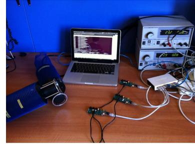
(c) Laboratory testbed using the channel emulator with SUNSET running on different hardware platforms.
