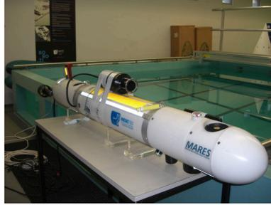
(b) MARES AUV with acoustic modem.
