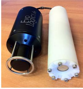
(a) Underwater monitoring node: Acoustic modem and measurement probe.
