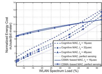
Fig. 6. Energy Cost with respect to WLAN Load for various channel detection times, with perfect sensing schemes for comparison.
