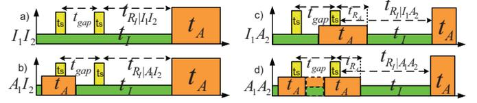
Fig. 2. Spectrum status cases at the time of the sensing measurements.
