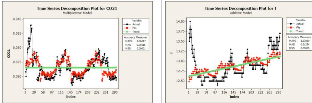
Figure 4. Graphs show an example of the time series decomposition for CO<sub>2</sub> (left) and temperature T (right) applied to a data subset collected in the Northern Adriatic sea. Both for T and CO<sub>2</sub> the two graphs show a seasonal component of 84 measures (14 days). Note that CO<sub>2</sub> graphs do not show any trend while all the temperature graphs highlight an increasing trend in the monitoring period.
