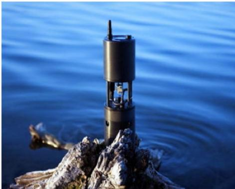
Figure 1. SAMI sensor for  $p\text{CO}_2$  measurement.
