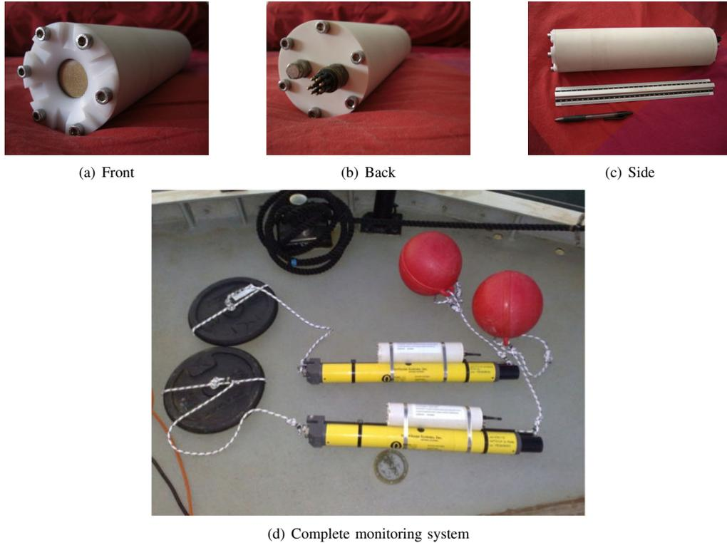
Figure 3. Underwater measurement probe.
