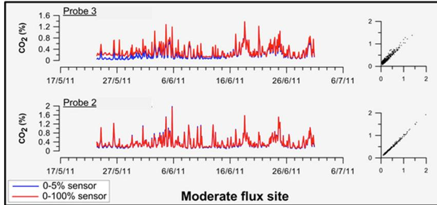
Figure 5. Dissolved  $\text{CO}_2$  concentrations (reported as  $\text{pCO}_2$ ) are given for the two probes deployed at the moderate  $\text{CO}_2$  flux site (probe 3 above, probe 2 below). Note that in each time series graph data is plotted from the two  $\text{CO}_2$  sensors in each probe (red and blue lines), and that the excellent correlation between these two sensors is illustrated in the X-Y scatter plots to the right.
