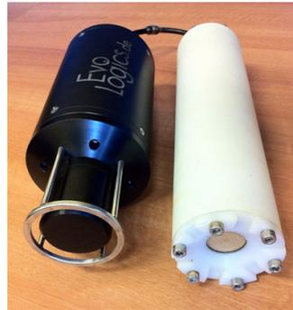
Figure 7. Underwater monitoring node: acoustic modem and measurement probe with the Gumstix inside the PVC housing.
