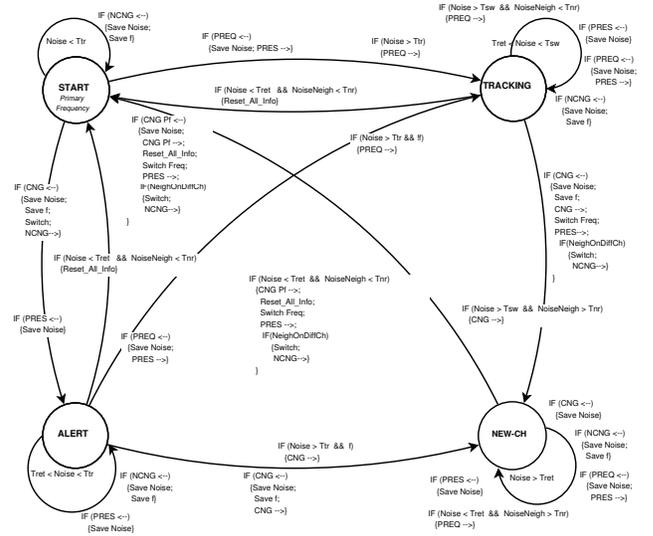
Figure 2: State diagram for the NAMAC protocol.
