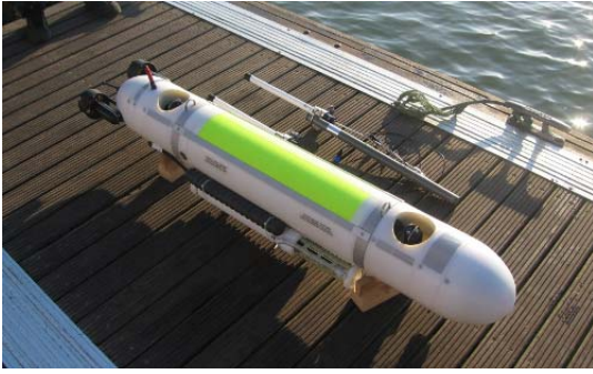
Figure 1: The MARES AUV with an externally mounted Conductivity, Temperature and Depth (CTD) sensor.
